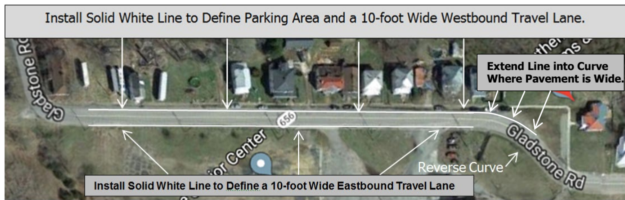
Figure 2: Gladstone Route 656 Proposed Pavement Marking Improvements
